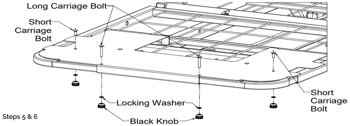
5. Align Deck Extension Pan holes with foot deck foot-end holes as shown above.
