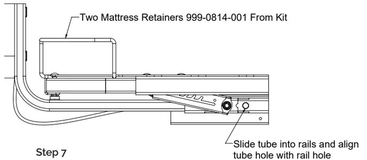
**Note:** In order to allow footboard mounting tubes to align properly and slide freely, only tighten footboard screws securely after footboard mounting tubes have been reinstalled and pinned into mainframe.
