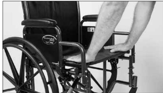
2. Use both hands to push down with even pressure on seat tubes and seat upholstery on insides of wheelchair, as shown at above left, until the seat rails are fully seated, as shown at above right. **Do not place any fingers or parts of your hand under the seat rails.**
