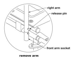
▲ WARNING: Ensure arm release is locked in place before occupying or operating wheelchair.
