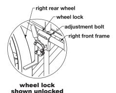
4. Use an M10 wrench to tighten the adjustment bolt and engage the wheel lock to check the fit. The wheel lock should indent the tire at least 3/8".
