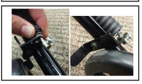
**6.** Make sure the brake lever is NOT in the locked position. While supporting the cable with the pliers, loosen the locking screw on the brass cable stop.
