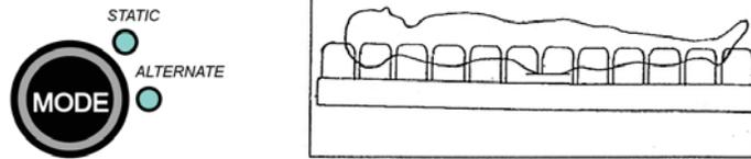
Press the front panel MODE button, shown at above left, to select STATIC mode. Adjust the Comfort Control by pressing the front panel SOFT / FIRM button to achieve the optimum patient comfort.
