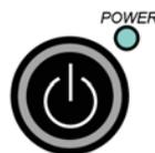
1. Press and hold the front panel POWER button (shown above) for one second — the POWER LED will now illuminate green indicating that the pump is operating.
