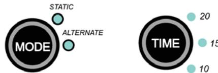
Press the front panel MODE button to select ALTERNATE mode and enable the two-one alternate function. Adjust the Comfort Control by pressing the front panel SOFT / FIRM button to achieve the optimum patient comfort. The ALTERNATE time cycle can be adjusted by pressing the front panel TIME button, shown at above right. The time can be ten, fifteen, or twenty minutes.
