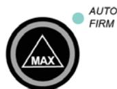
2. Press the front panel MAX button (shown above) for AUTO FIRM inflation — comfort level and therapy lights will not illuminate during MAX inflation. Allow time for full mattress inflation. After the mattress is fully inflated, the patient can be transferred to the mattress. **Note: the mattress can be inflated while a patient is lying on it.**
