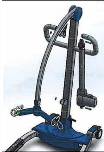
5. Attach the actuator to the lifter with cotter pins as shown above.
