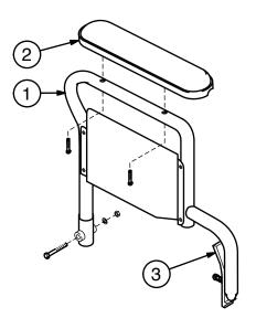
Arm, flip-back fixed-height, pair (includes right and left arm with mounting hardware, side panel, and latch; does not include arm pad)
