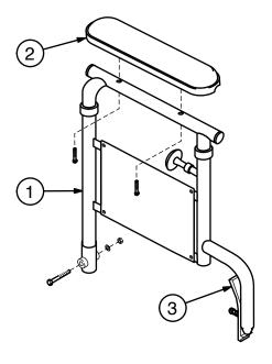
1 Arm, flip-back adjustable-height, pair (includes right and left arm with mounting hardware, side panel, and latch; does not include arm pad)
