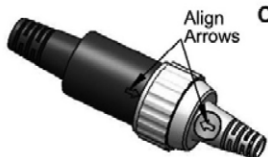
DETAIL B: ENSURE LOCK END CAPS ARE SCREWED ON SECURELY
